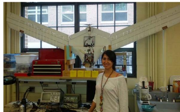
The airfoil cross-section is positively cambered for good lifting characteristics at low angles of attack. The center of gravity is ahead of the aerodynamic center, providing static stability in the longitudinal axis. Lateral stability is provided by the winglets.
