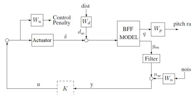
Figure 4: Interconnection for controller synthesis
