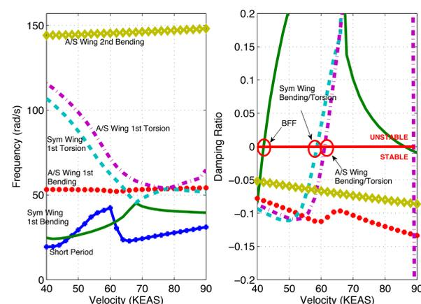
Figure 3: Velocity/frequency/damping plot
